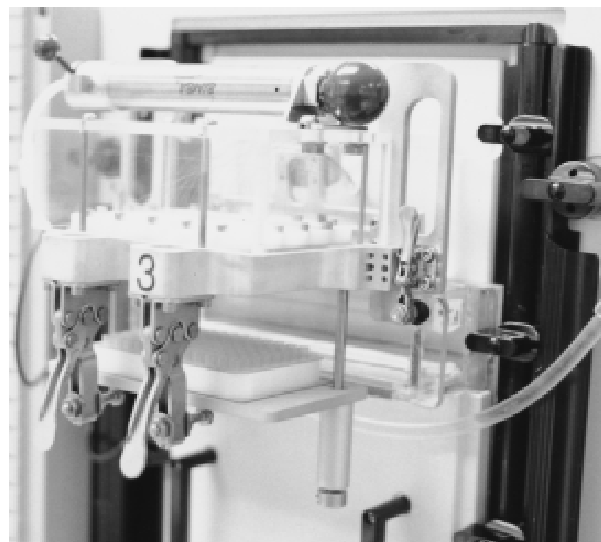
Figure 3 A 72-lane gel loader mounted on the upper buffer tank and the gel cassette of the PE/ABI 377 sequencer. The Genome Sequencing Center upper buffer tank is shown mounted on the PE/ABI instrument. The gel-loading device is attached onto the upper buffer tank.
