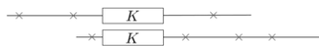
Figure 1. Illustration of the alignment of two reads by identifying a common k -mer in the overlap. The boxes labeled by K denote a common k -mer between the two reads. The symbol \times denotes a sequencing error that would preclude a common k -mer from occurring in the immediate area. However, as long as the error rate is low enough and the overlap is sufficiently long, a common k -mer will exist with high probability.
