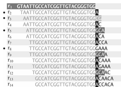
Figure 2. Removing transitive edges. A read r_1 with 13 other reads ( r_2 \dots r_{14} ) that overlap on its right end side are shown in the form of a multiple alignment. The overlaps that do not correspond to transitive edges are indicated with a black dot. The transitive edges removal procedure consists in discarding the overlaps that are already overlapped by another read involved in a larger overlap with r_1 . For example, the reads r_4 , r_6 , r_7 , r_{10} , r_{11} , r_{13} , and r_{14} are overlapped by r_2 ; they are therefore removed from the set of overlapping reads of r_1 . Same principle is applied to the reads r_3 , r_5 , and r_8 . This example is issued from a real data set of reads of 26 bases.
