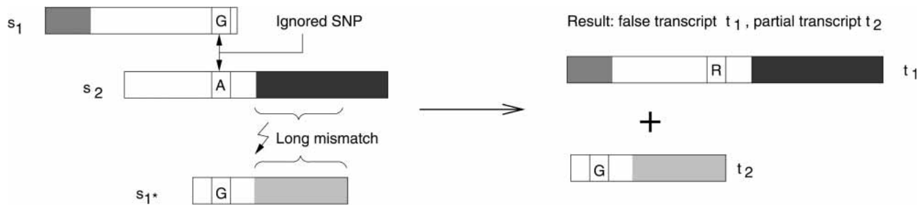
Figure 1 Example of a misassembled transcript when SNPs are disregarded. Assembly of three input sequences are shown at left ; the resulting transcripts of this assembly are shown at right . The three sequences s_1 , s_{1^*} , and s_2 contain different homologous parts, represented by the different shades of gray, and exactly one SNP position. A normal assembly algorithm will assemble first s_1 , then s_2 (because of the long overlapping alignment in the white part), and then might try to align s_{1^*} , but fail because of the large mismatch. The SNP position with G in sequence s_1 and A in s_2 is treated as typical noise in the alignment algorithms and ignored. The resulting transcript sequences are therefore wrong, as they do not represent the sequences found in vivo: t_1 is a mix of two transcripts and does not code a true protein.
