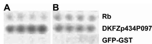
Figure 7 In vitro phosphorylation of arrayed proteins. Purified proteins were arrayed in quadruplicate on glass slides, and incubated with different protein kinases in the presence of [\gamma\text{-}^{33}\text{P}]\text{ATP} . Rb is the retinoblastoma protein (Lee et al. 1987), which served as positive control. GFP-GST is purified fusion protein of GFP with a GST-tag, which should not be phosphorylated by the kinases. The protein from cDNA DKFZp434P097 was expressed as a fusion protein with the C terminus of GST. (A) The array was incubated with CDK2/cyclin E kinase. (B) The array was incubated with p42 MAPK kinase.
