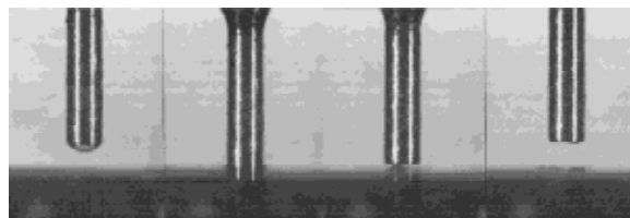
Figure 1 Detailed illustration of the liquid transfer by a spotting pin. Close-up view of one pin spotting a PCR product onto a glass slide. In the outer-left picture, the 250- \mu m pin tip end is loaded with a 2-nL droplet. The left picture shows the actual spotting process onto the epoxysilanated glass surface. In the right picture the pin goes up again, showing that the liquid's surface tension is present and does not allow the immediate delivery of the whole droplet, which might be one reason for the well-known doughnut effect. The outer-right picture finally shows pin and glass surface after liquid delivery. It is obvious that a tiny amount of DNA solution is still sticking to the pin, which requires careful cleaning procedures prior to the next spotting run.
