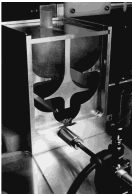
Figure 9 Capillary dispenser. Capillaries (A) are shown in the bottom of the trough.
