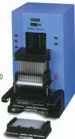
*The Hydra-96 and special plate positioner is used for quick dispensing of reagents into the reaction chambers of CyclePlate-384 and -192.*
