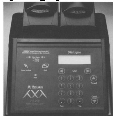
MJ Research's newest thermal cycler, the PTC-200 DNA Engine™, brings new capabilities to the field of DNA sequencing and amplification. This speedy Peltier instrument has a temperature range of -5° to 105°C, and it features a swappable block format for
