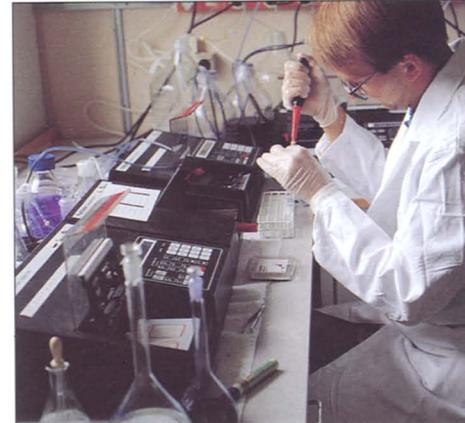
Carefully controlled electrophoresis at different temperatures on different electrophoretic gel media is essential for detecting the maximum number of mutations by PCR-SSCP analysis. PhastSystem™ and PhastGel® media combine these attributes in a cost efficient and easy-to-use format.
