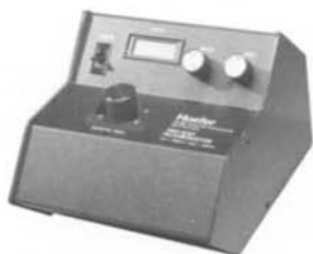
TKO 100 Mini Fluorometer Measures DNA concentrations before amplification to standardize reaction conditions and after amplification to evaluate the yield.
